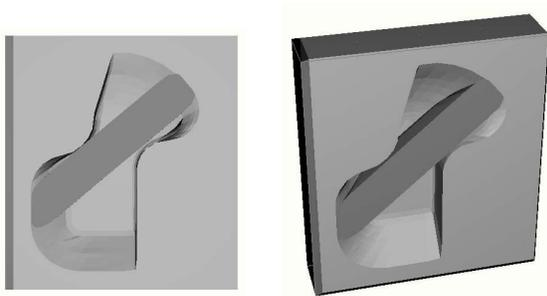
Figure 1. CFD model, hinge geometry.
