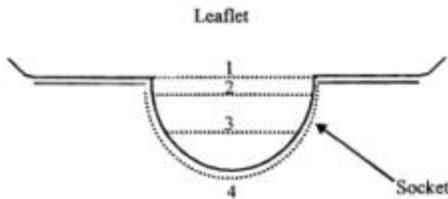
Figure 2.2. Cut locations in socket area.
