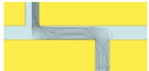
Streamline analysis for charged particles released within a channel of a microfluidic chip for electrophoretic movement of charged compounds.
