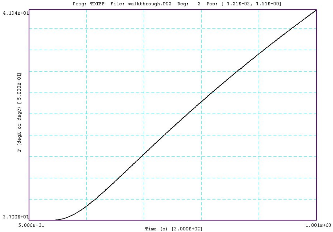
Figure 4. Plot of the time-variation of temperature at the probe position created by the Probe program.
