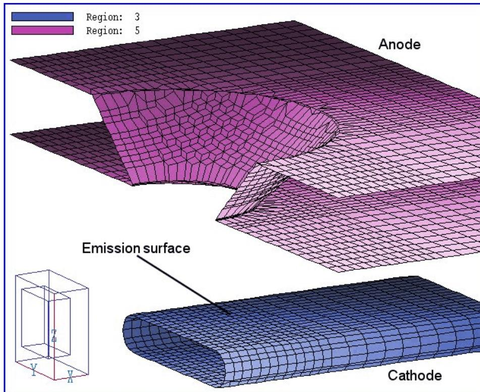
**Figure 2.2.** Anode and cathode shapes – ribbon example.
