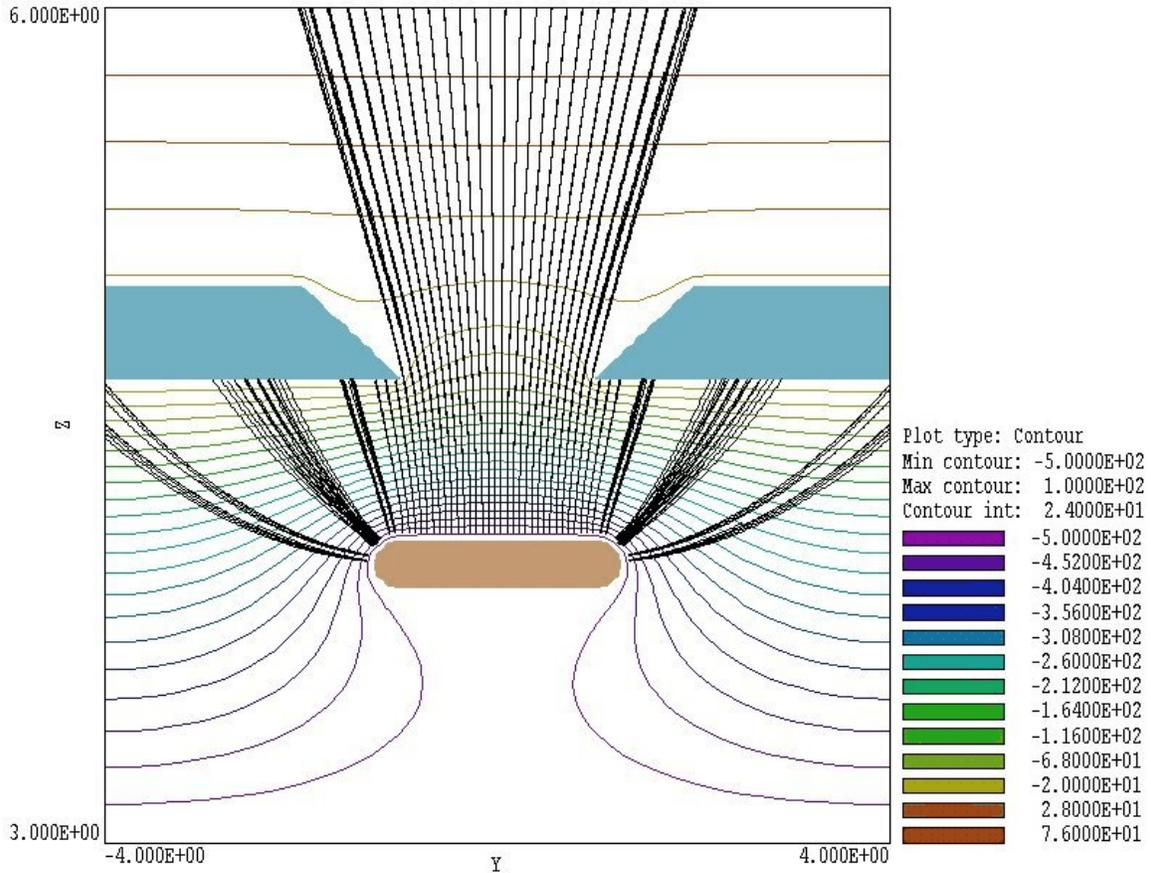
**Figure 2.5.** Two-dimensional plot of electrostatic equipotential contours and projected orbits, example *ribbon*.
