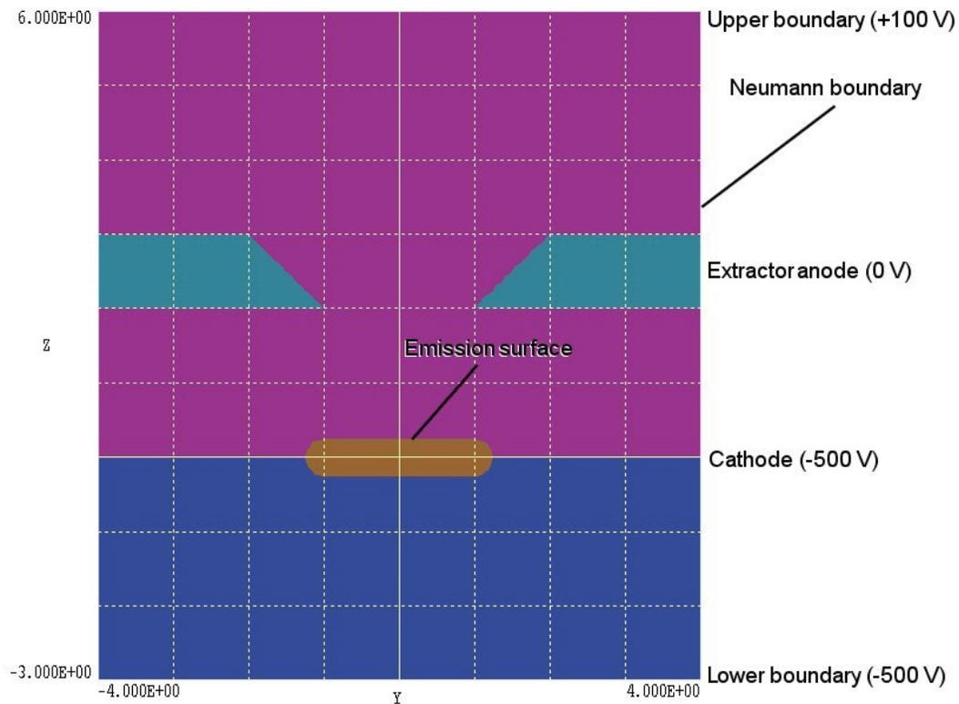
**Figure 2.3.** Cross-section of the geometry of example `ribbon.min` in a plane normal to  $x$  at  $x = 0.0$ . Lower vacuum volume: region 1 (blue). Upper vacuum volume: region 2 (violet). Cathode: region 3 (orange). Anode: region 5 (green).
