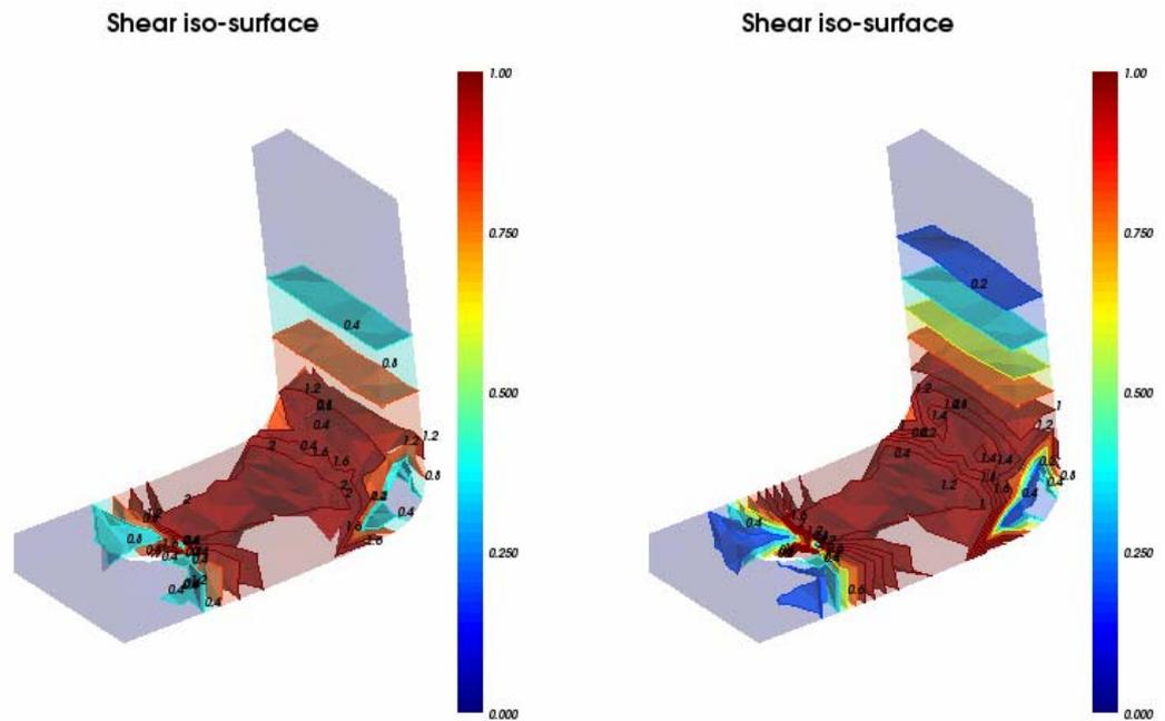
Figure 5.7.1.5 Display the shear iso-surfaces of the L-shape steel board
