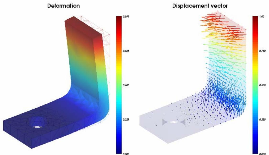
Figure 5.7.1.2 Display the deformation and displacement vector of the L-shape steel board
