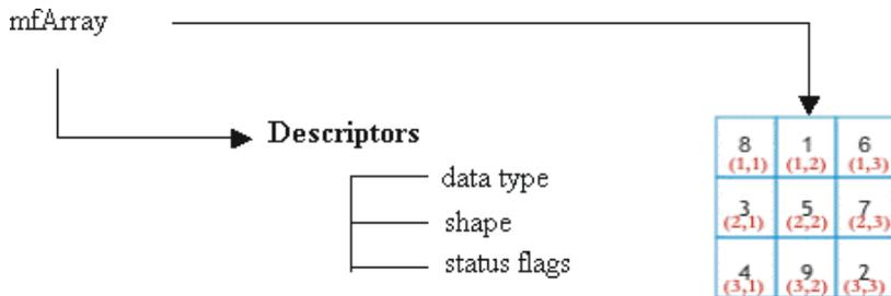
Figure 2.1.1 Structure of the `mfArray` data object
