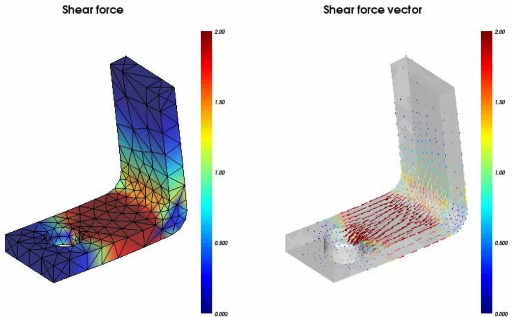
Figure 5.7.1.3 Display the shear force and the shear force vectors of the L-shape steel board
