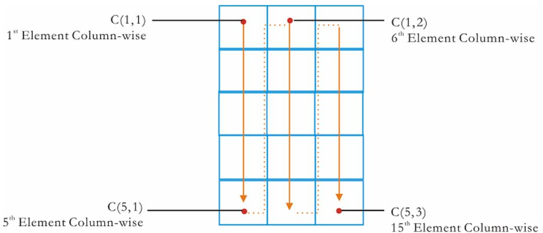
Figure 2.1.3 Element ordering in an mfArray data object
