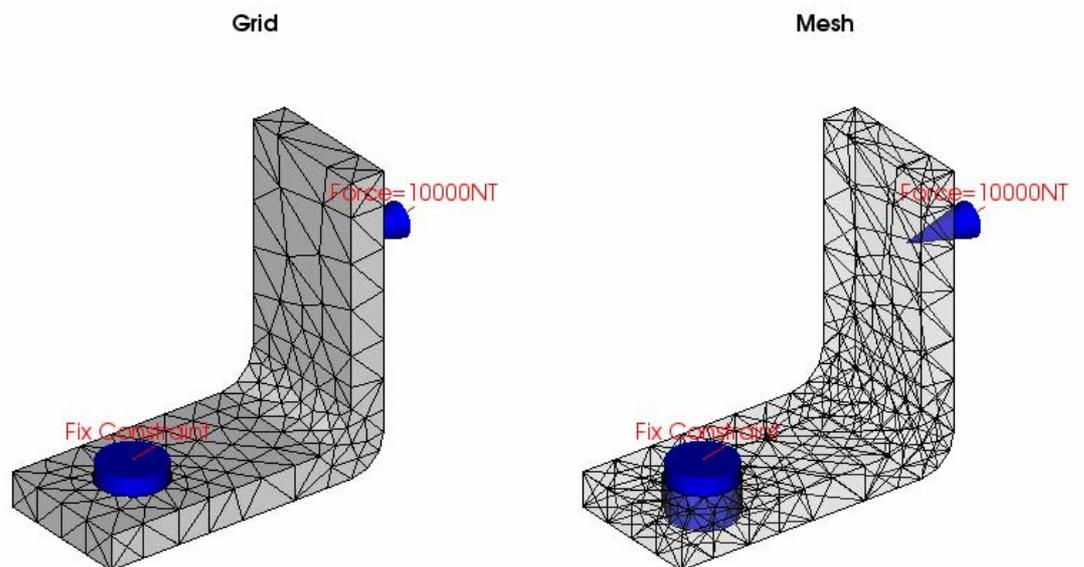
Figure 5.7.1.1 Display the grid and mesh plot of the L-shape steel board
