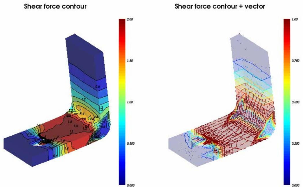
Figure 5.7.1.4 Display the shear force contour and vector of the L-shape steel board
