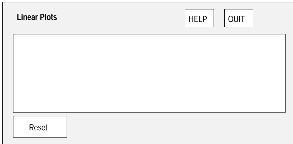
Figure 10: Above is a very simple GUI for a "superplot" program. The GUI for "superplot" contains a workspace, an action button, a help button, and a quit button. Below is the UIS file that describes the "superplot" GUI.
