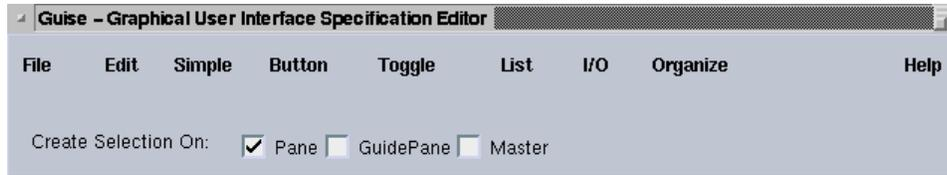
**Figure 1:** The guise GUI specification editor allows the user to input and display an existing UIS file, or to create a new one. Selections may be added, old selections deleted, or existing selections changed.
