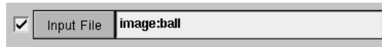
Figure 2: An optional input file selection has the optional box to the left. A checkmark is displayed when the option is selected.
