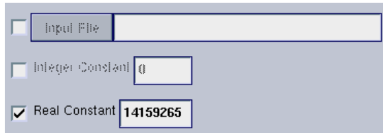
Figure 36: A mutually exclusive group containing an input file, an integer, and a float. Currently, the "Real Constant" float parameter is selected for use; the other two selections are desensitized to emphasize that they will not be used.
